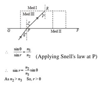
When the refracted ray PR meets the boundary DE, it is travelling from a denser medium to a rarer medium. Therefore the ray will be totally internally reflected at DE if its angle of incidence r is more than the critical angle for med III and I.
