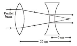
From the diagram it is clear that the focus of both the lenses should coincide as shown in the diagram.
