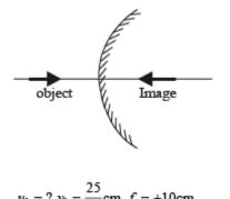
$$\frac{1}{v_1} + \frac{1}{u_1} = \frac{1}{f}, \quad \frac{3}{25} + \frac{1}{u_1} = \frac{1}{10} \therefore u_1 = -50 \text{ m}$$
