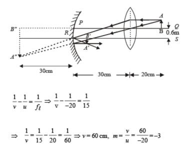
The image is formed to the left of the lens, real, inverted and three times the actual size (3.6 cm in height below PQ).
