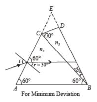
(a) The rays of wavelength  $\lambda_0$  incident at any angle on the interface BC will pass through without bending, provided the refractive indices  $n_1$  and  $n_2$  have the same value for the wavelength  $\lambda_0$ . Equating the expressions of  $n_1$  and  $n_2$ , we get
