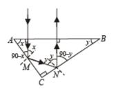
Let y be the incident angle of the ray on face CB. For total internal reflection
